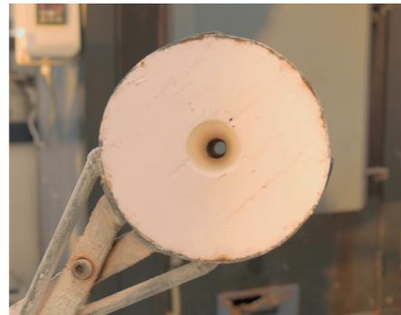
“Through the chimney effect, CLEANFLOW allows an easier and natural flow from the top of the slags and combustion gas caused by wax pouring, resin burning or use of similar materials for the creation of the tree”.
